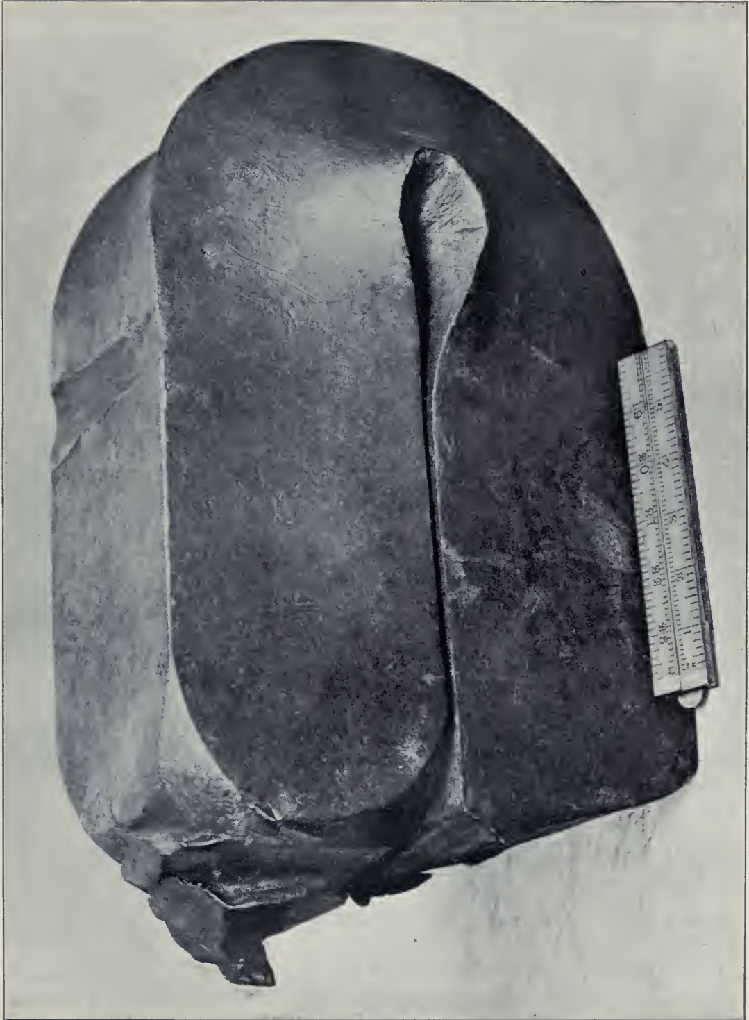
FIG. 69. BESSEMER STEEL GUN TEST-PIECE, SHOWN AT THE MEETING OF THE INSTITUTION OF MECHANICAL ENGINEERS AT SHEFFIELD, 1861
