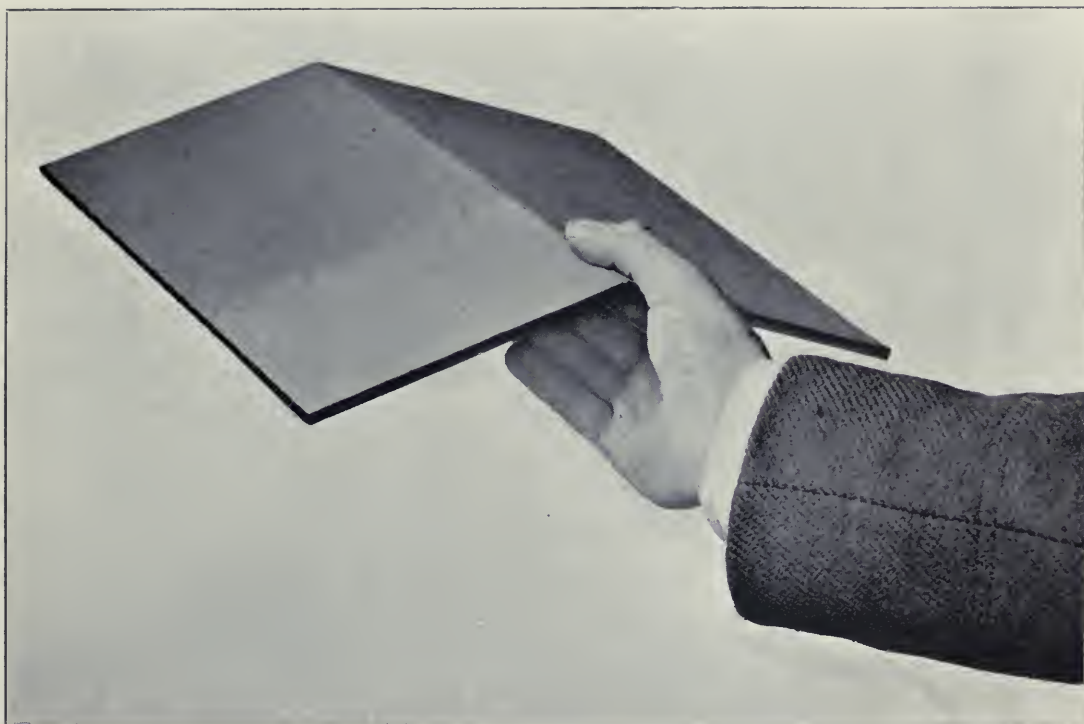
FIG 72. ALLEGED FAULTY BESSEMER PLATE, 1875
