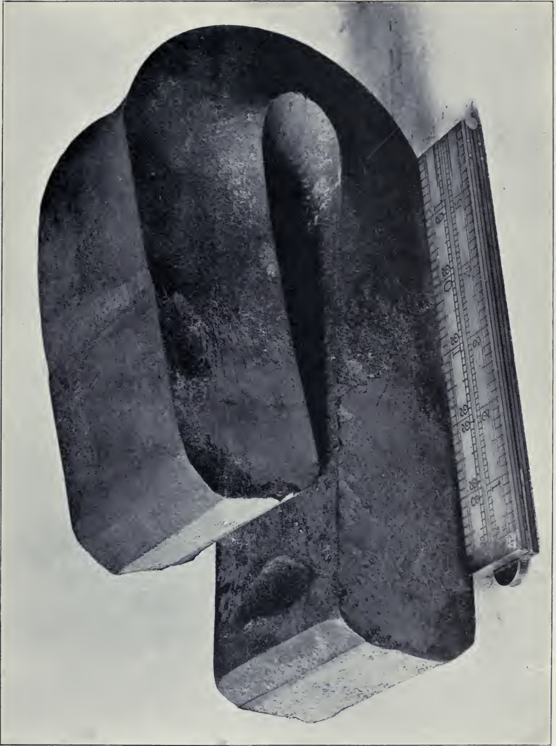
FIG. 70. BESSEMER STEEL GUN TEST-PIECE, SHOWN AT THE MEETING OF THE INSTITUTION OF MECHANICAL ENGINEERS AT SHEFFIELD, 1861
