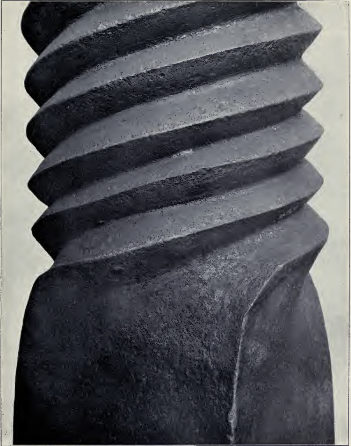
FIG. 57. SQUARE BAR OF BESSEMER METAL TWISTED COLD, AND SHOWN AT SHEFFIELD, 1861
