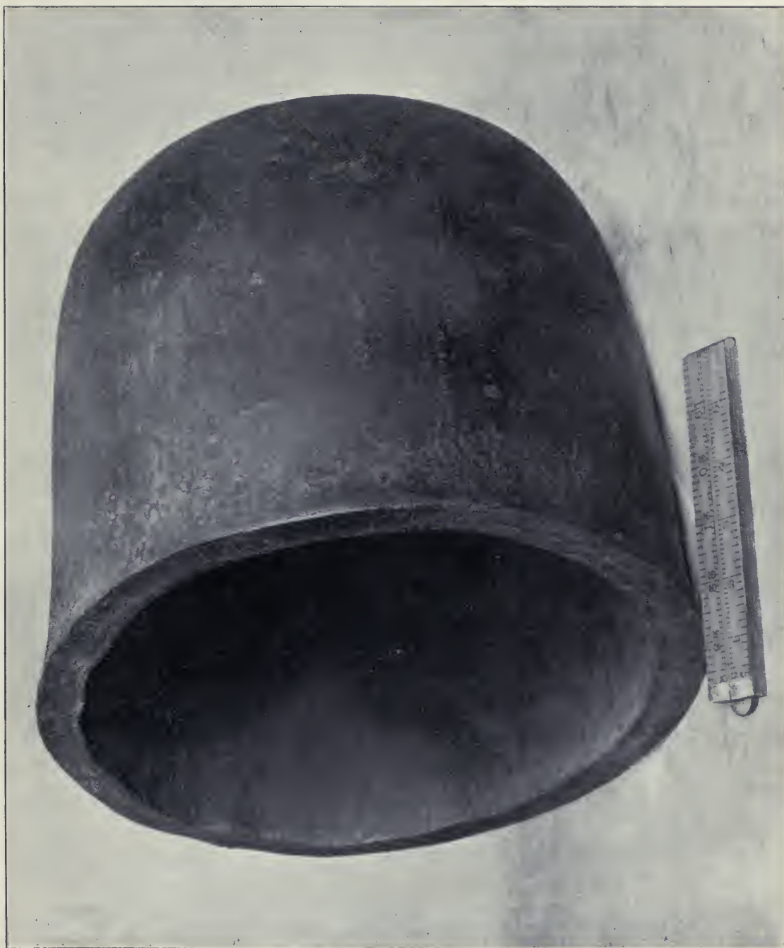
FIG. 56. BESSEMER STEEL BOILER PLATE PRESSED INTO A CUP, 1861
